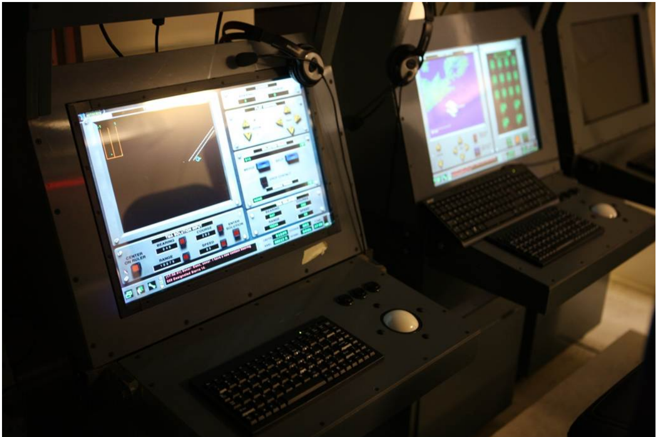
Figure 4: The target motion analysis and fire control stations inside VCEL.
